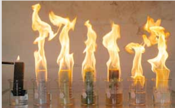
Beakers of oil with insulation materials being used as wicks. Only FOAMGLAS® (left-hand side) prevents wicking fires.
